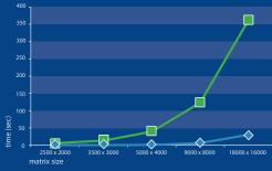
Scaling of Out-of-Core SVD as a Function of Matrix Size
